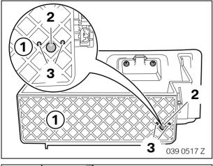
All holes must be drilled precisely as shown in the illustration.
