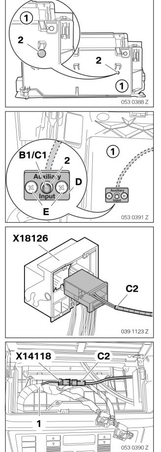
All holes must be drilled precisely as shown in the illustration.
