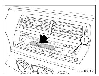
16. Route Auxiliary Input Cable (2) from radio harness (1) down through position indicated by black arrow.
