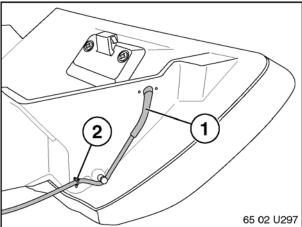
20. Fasten Auxiliary Input Cable (1) to side of glovebox by routing cable tie through holes (2). Remove excess material from cable tie.
