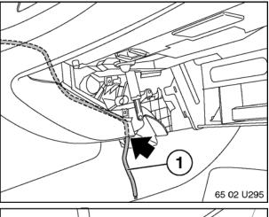
18. Route Auxiliary Input Cable (1) down through dashboard through position indicated by black arrow.
