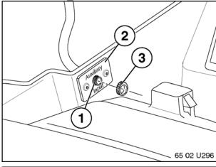
19. Insert Audio Jack (1) into faceplate (2) and secure with provided nut (3).
