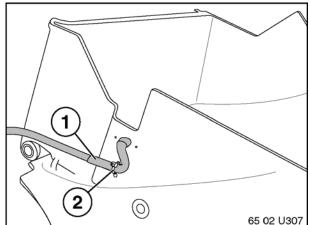
17. Route Auxiliary Input Cable (2) from radio harness (1) down through position indicated by black arrow.
