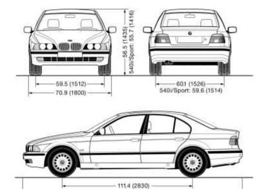
All dimensions are given in inches (mm). Min. turning circle dia.: BMW 528i 37.1 ft (11.3 m), BMW 540i 37.4 ft (11.4 m)
