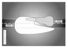
The xenon lamps light up the side and front areas of the vehicle with significantly more brightness and uniformity then the traditional halogen lamps.
