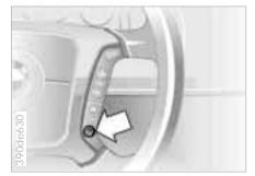
To activate and cancel the steering wheel heater, press the button (arrow) with the ignition key in position 2.
