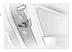
Insert the key into a rear door lock and turn it outward:
