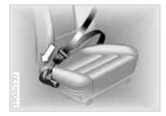
The safety belt tensioner responds to severe frontal collisions by tightening the belts to ensure that occupants remain firmly positioned in their seats. A gas-pressure system retracts the buckle assembly to tension the shoulder and lap belts within fractions of a second. This reduces the tendency to slide under the lap belt.
