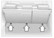
If you use a child restraint system with a tether strap, three additional tether anchorage points (refer to the arrows – the illustration shows the sport wagon) have been provided. Depending on the location selected for seating in the rear passenger area, attach the tether strap to the corresponding anchorage point to secure the child restraint system. Remove the cover first on the middle location.
