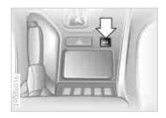
You can operate the central locking system with this button when the driver's door is closed. With this button, only the doors, the luggage compartment lid/tailgate and rear window are unlocked or locked. The anti-theft system is not activated. Also, the fuel filler door remains unlocked to allow refueling.
