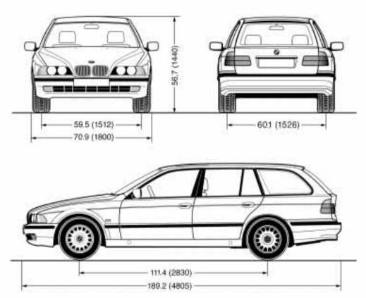
All dimensions are given in inches (mm). Min. turning circle dia.: BMW 528i 37.1 ft (11.3 m), BMW 540i 37.4 ft (11.4 m)
