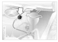
5 Then connect the negative terminals. Attach the cable to either the support vehicle's negative battery terminal, or to a suitable ground on its engine or bodywork. Then connect the other end of the cable to a ground on the engine or body of the vehicle which is to be started. There is a special nut on the strut dome of your BMW; refer to the arrow in the illustration.
