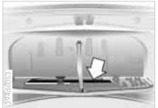
The hazard warning triangle is quickly available, stored in the onboard tool kit mounted on the inside of the luggage compartment lid (tailgate).
