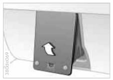
4 Use the magnetic retainers to attach the cover panel to the upper surface (metal surface below rear tray) of the luggage compartment.
